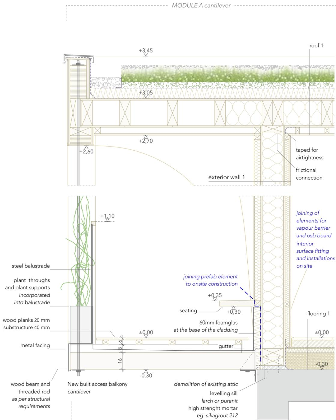
Detailed Section and Elevation Cantilever 1:20
