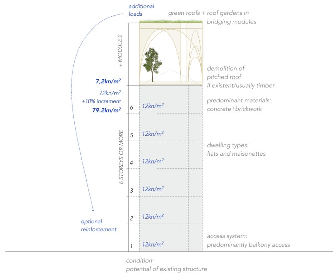
Following these estimations, the additional structure can accommodate the proposed one or two storey timber frame constructions (~4kN/m<sup>2</sup> or 6,5kN/m<sup>2</sup>) with extensive green roofs above the flats. The bridging units in between allow for the provision of intensive vegetation including small trees.
